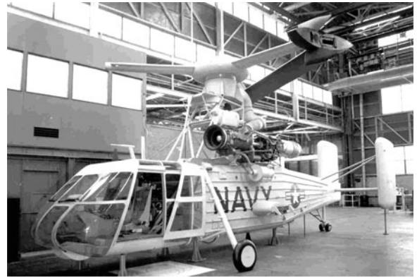
Fig. 15. XHCH-1 mockup (showing rotor fold).
