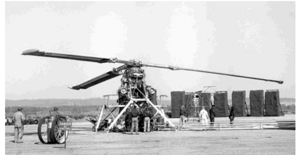
Fig. 16. Full-scale XHCH-1 rotor hot-whirl rig.
